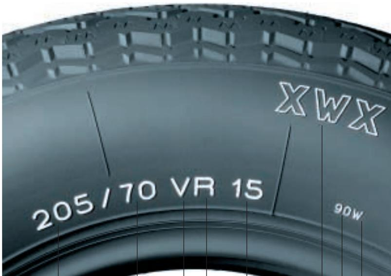
Tyre width (mm)      Aspect ratio      "R" for Radial      rim diameter      load index      tread pattern      maxi speed 270 km/h
